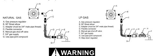
When installing the pressure regulator - remember it can only handle 1/2 PSI. In every LPG installation, you have high source pressures, ranging from 20 PSI to 100 PSI. If the high pressure gas line from the LPG tank is directly connected to the unit without the proper step-down regulator, it will rupture the diaphragm in the valve, rendering it useless.
