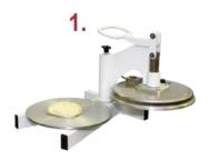
1. After allowing upper platen to reach desired temperature, place pre-portioned ball of dough in center of platen.
