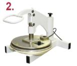
2. After setting time and desired thickness, swing upper platen over dough ball and pull down the handle until it locks into position. Using both hands, pull up the handle.
