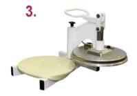
3. Remove your crust from the platen and place on screen, disc, or pan (top of crust on press becomes bottom). Now you are ready for makeup and baking.
