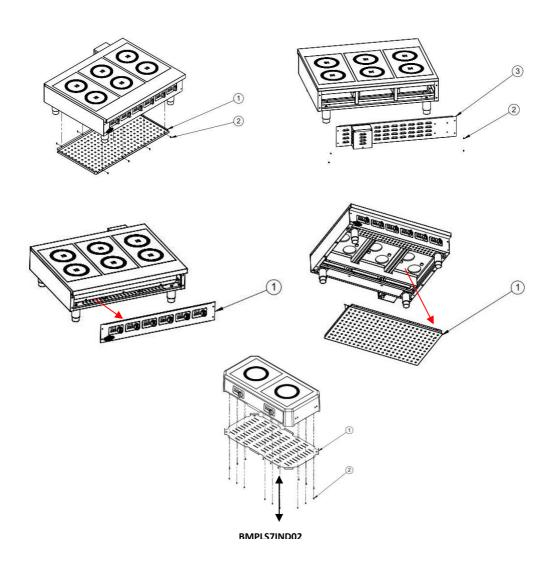
We recommend cleaning the bottom panel and front panel (No 1) and back panel (No 3) at least every year. Please remove and remove the screws (No 2) with screwdriver, clean with wet cloth. (Do not use bleach and abrasive chemicals)
