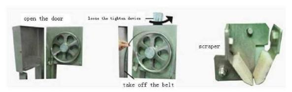
Also it can use the wet slip and hot water and scour to wash the main spare parts ,belt and protective device. Finally, please wipe off all water from the machine by dry cloth.
