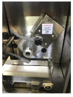
The BakeMax BMCCD01 Countertop Continuous Dough Divider divides dough fast and efficiently. Comes with a 33lb dough hopper and power outfeed belt. This unit is great for pizza, bread, and other types of dough (avg. humidity of 55%). This unit has a production output of 500-2000 pieces per hour, depending on the operator.
