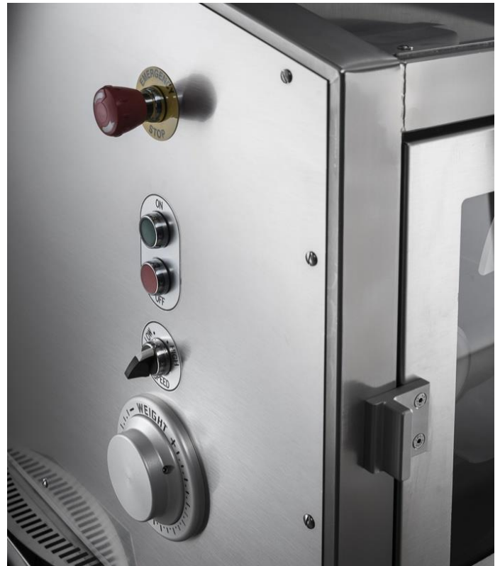
Emergency Stop, On / Off Buttons Speed Control and Weight Control
