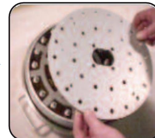
Figure 7: Now lift the Plug Plate, exposing the Stems.
