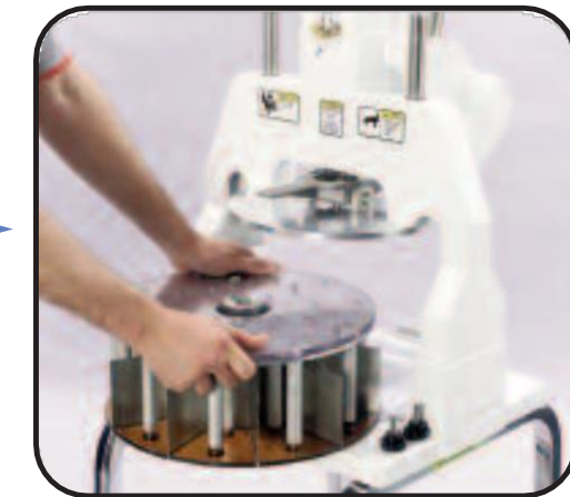
Figure 4: Return the Handle to the upper position and remove Head Assembly for cleaning or interchange with Optional Head Assembly.
