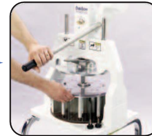
Figure 3: While holding the Handle down with one hand, use your other hand to rotate the Head Assembly 1/4 turn until the Head Assembly releases.
