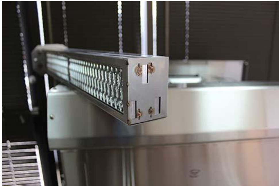
Filter Tray Notches for Engaging Switches (All 3 filters must be installed correctly to engage switches)
