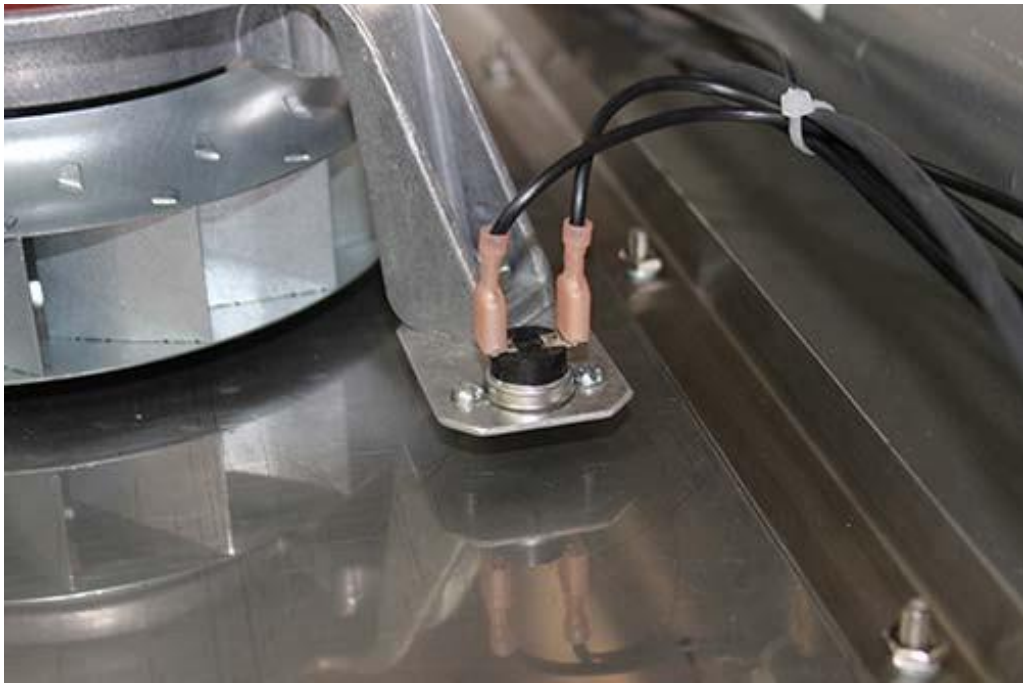
Top Oven Compartment Thermostat set to 145°F
