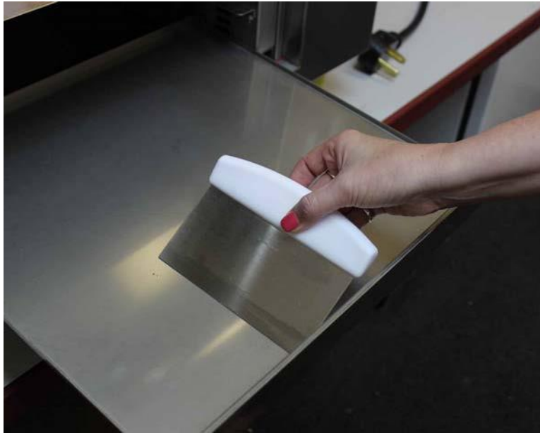
Scraping the Drip Tray to Clean
