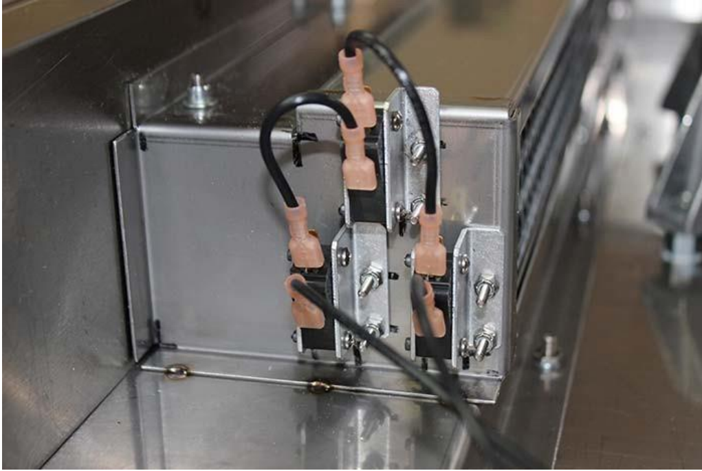
Interlock Filter Switches
