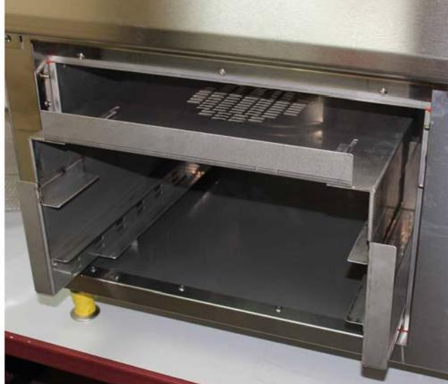
Air Plenum Pulled Out of Oven Chamber
