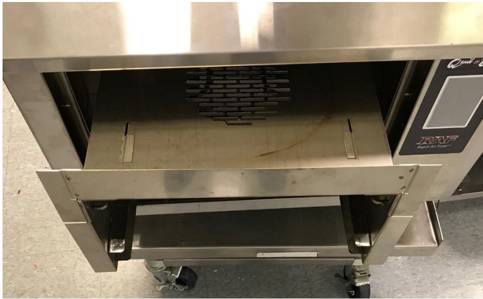
Air Plenum Pulled Out of the RAF
