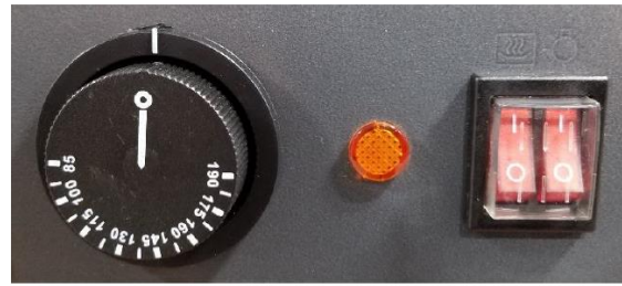
Manual Temperature Control
